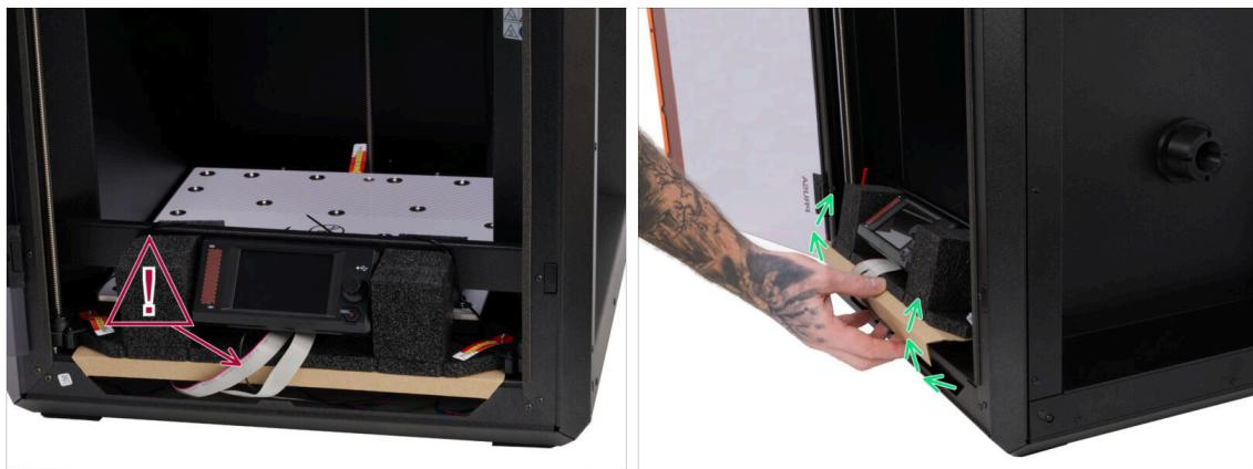
⚠ In the next few steps, make sure not to damage the LCD cables.
