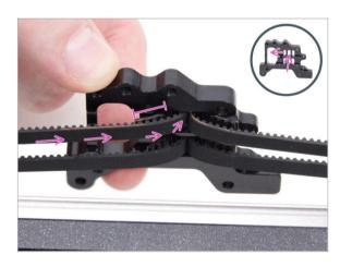
Push the end of the belt through the middle hole to the left hole in the upper row of the Nextruder holder leave 4-5 teeth sticking out.
