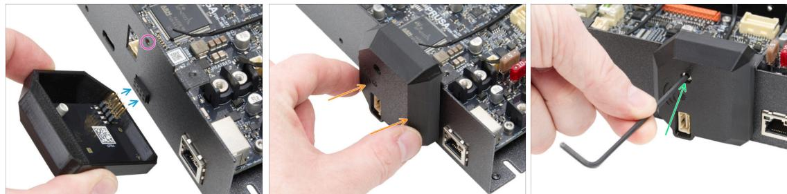
**⚠️ Be very careful when handling and connecting the ESP module to avoid bending and damaging the pins.**
