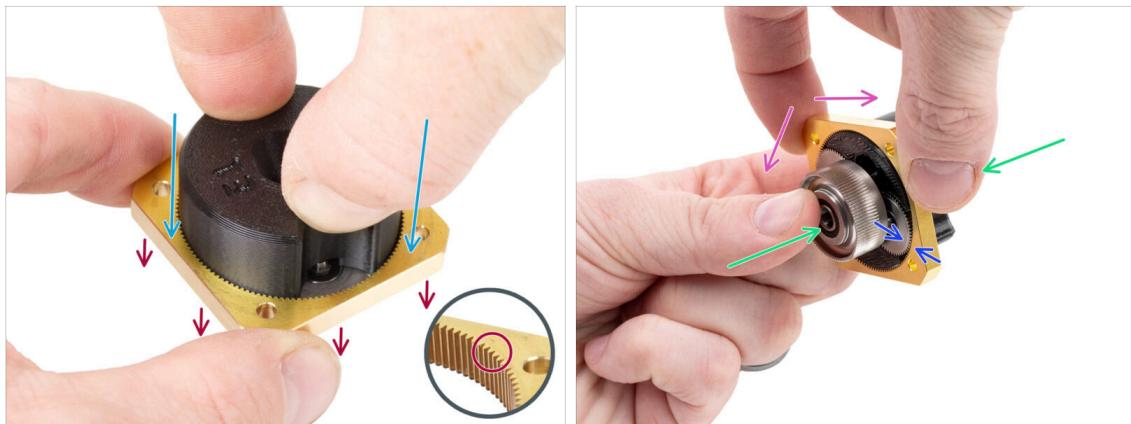
**⚠ Do not assemble the gearbox without the PG-assembly-adapter.** This tool is intended to ensure that the gears are correctly fit together.
