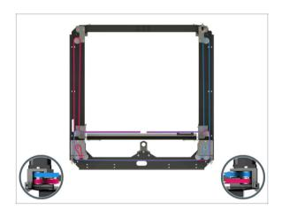
Before proceeding, recheck the belt routing according to the illustration.
