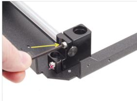
Focus on the front left holder (now on the right) and secure the rod by tightening the screw in the holder.
