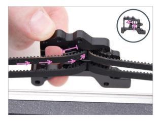
Push the end of the belt through the middle hole to the left hole in the upper row of the Nextruder holder leave 4-5 teeth sticking out.
