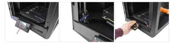
Gently lift the xLCD assembly into the upward position.
