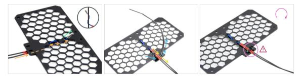
• Guide the thermistor cable under the grid. Thread it in the direction shown in the picture.
