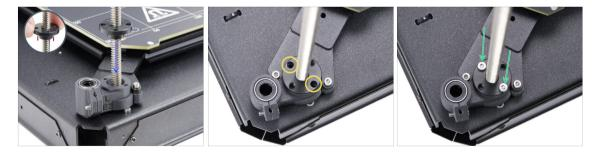
Manually thread the trapezoidal nut onto the left Z motor. Screw the nut all the way down until it seats into the plastic part.
