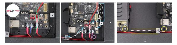
• Take one red cable leading from the PSU and connect it to the first left terminal slot on the xBuddy board using the 6/32" terminal screw. Tighten it firmly but gently.
