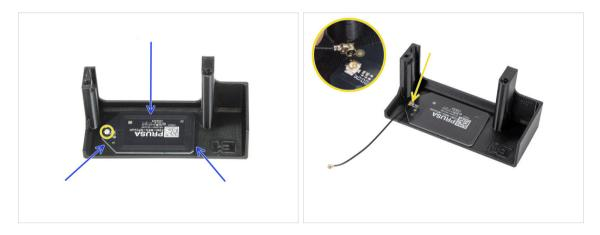
Stick the NFC coil onto the inner side of the El-box cover, approximately as shown in the picture.
