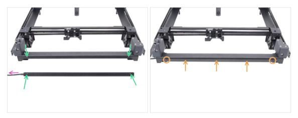
Take the white LED assembly and attach it to the front of the CoreXY assembly. Align the holes of both parts.
