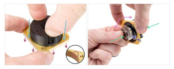
Do not assemble the gearbox without the PG-assembly-adapter. This tool is intended to ensure that the gears are correctly fit together.
