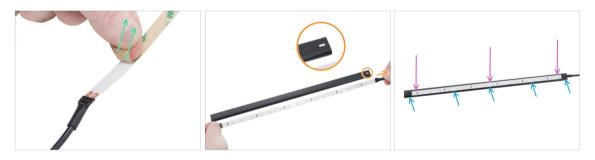
• Carefully peel off the protective (paper) layer from the White LED strip.
