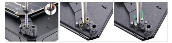
Manually thread the trapezoidal nut onto the right Z motor. Screw the nut all the way down until it seats into the plastic part.
