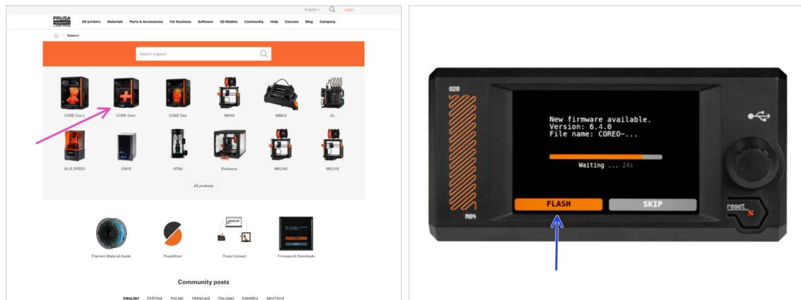
ⓘ All printers come with a USB drive containing the latest firmware. However, it is recommended to check and possibly upgrade the firmware version every few weeks.
