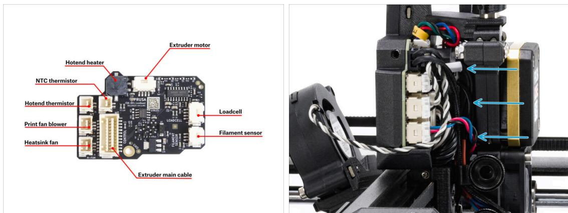
**⚠ Before covering the electronics, check the connection of all cables.**
