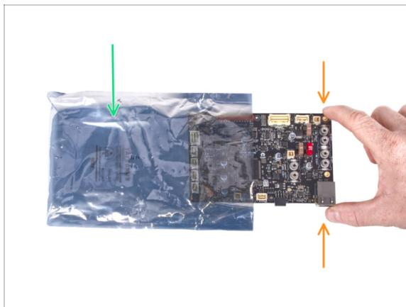
**⚠ WARNING:** Make sure to protect the electronics against electrostatic discharge (ESD). When possible, always unpack the electronics right before you need them.
