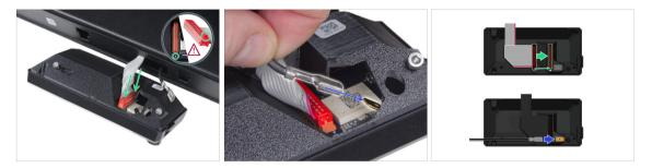
Connect the xLCD cable (gray cable with red connector) to the xLCD board on the back of the xLCD assembly. Do not pull on the cable!
