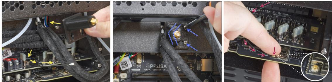
① This step is only for the printer, which has a Wi-Fi antenna on the back of the printer. If you have the **antenna on the side** of the printer, **proceed to the next step**.
