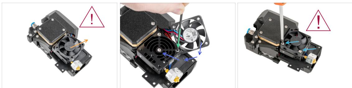
**⚠️** The heatsink fan is **still connected**, be gentle about the cables!
