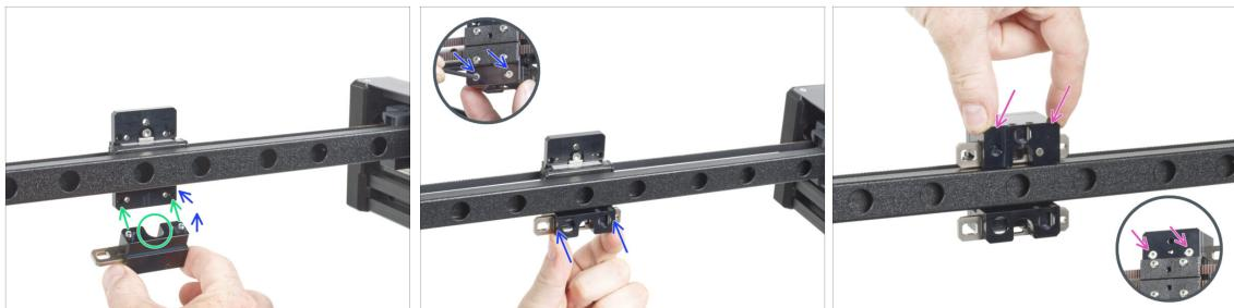
**⚠ Be careful that the springs and pins do not fall out when handling the parts.**
