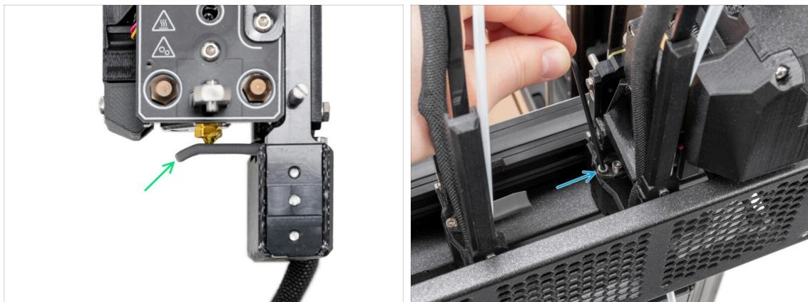
① Starting from May 2024, you may receive a gray nozzle seal. The assembly and functionality remain identical to the red one.
