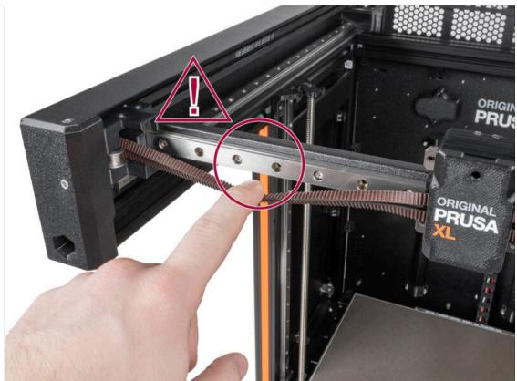
**⚠ CAUTION: Avoid direct skin contact with the lubricant used for the linear rails in this printer. If a contact occurs, wash your hands immediately. Especially before eating, drinking, or touching your face.**
