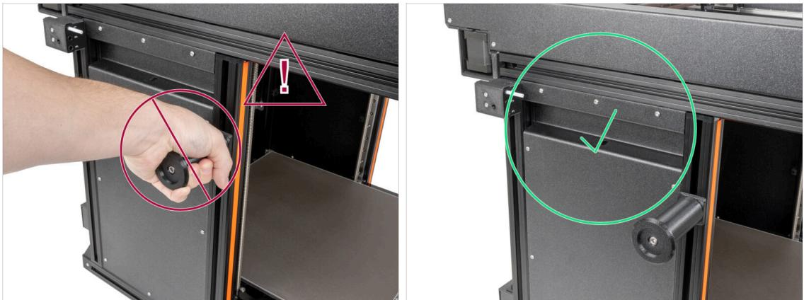
**⚠️ Never manipulate the printer by using the upper metal flanges. You can damage the LED lights hidden inside.**
