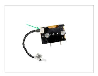
• Connect the tool-changer cable with the tool-changer.
