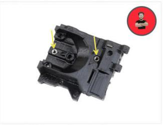
**● Insert two M3n nuts to the X-carriage-back.**
