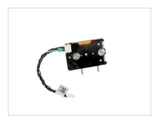
Connect the tool-changer cable with the tool-changer.
