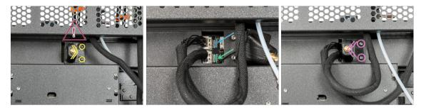
• Locate the Wi-Fi-antenna-holder (cover) on the rear of the printer.
