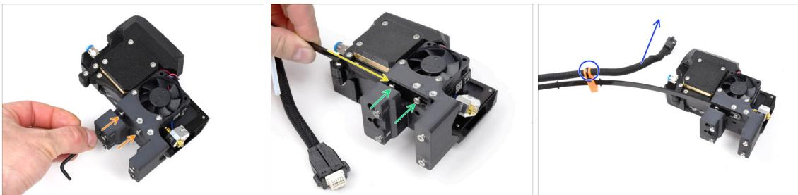
● Using the T10 key, loosen the marked two screws on the inside of the nextruder.
