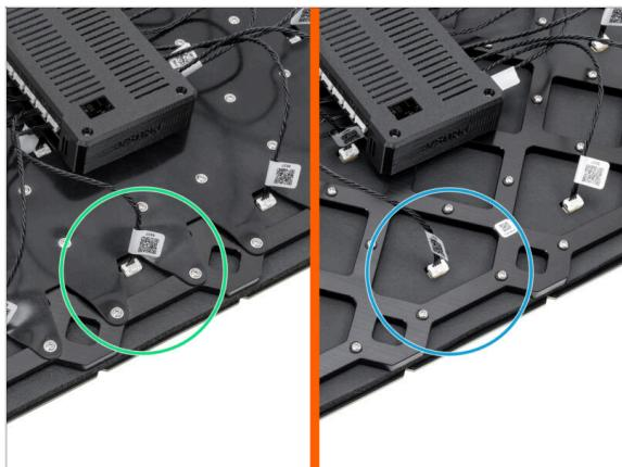
**i** Starting from April 2025, you may receive a new heatbed. The difference is the black rubber band on a back side of the heatbed.
