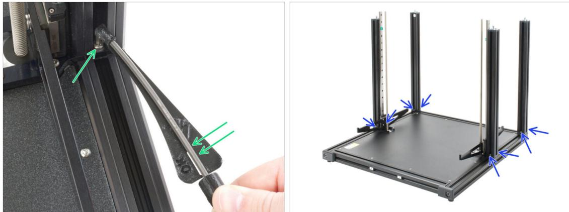
**⚠ Attention: Make sure that the Allen key is inserted ALL THE WAY into the screw. Do not overtighten the screws over the torque indicator scale!**
