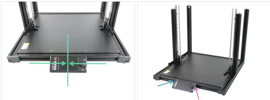
⚠ **Aligning the xLCD to the center is recommended or you can go slightly to the left side. Moving the xLCD to the right is not recommended as the cables won't be long enough.**
