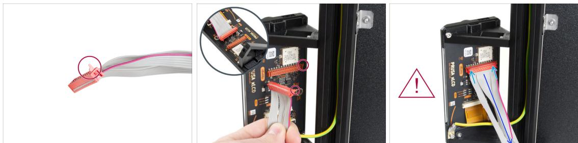
**⚠** The xLCD cable connector has a locking latch that has to face the red triangle near the xLCD connector.
