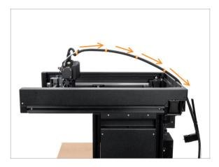
Guide the Nextruder cable bundle with the PTFE tube freely over the printer to its rear side.
