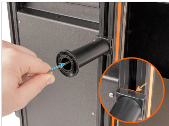
🟡 Attach the spool holder assembly to the M4nEs nut in the extrusion. Note that there is a protrusion on the spool-holder-mount, which must fit into the groove in the extrusion.
