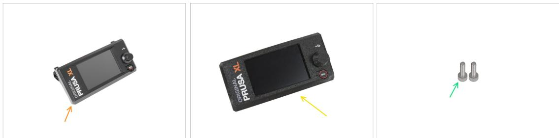
① Starting from September 2024, you may receive a new injection-molded xLCD. Check the photos and identify your version.
