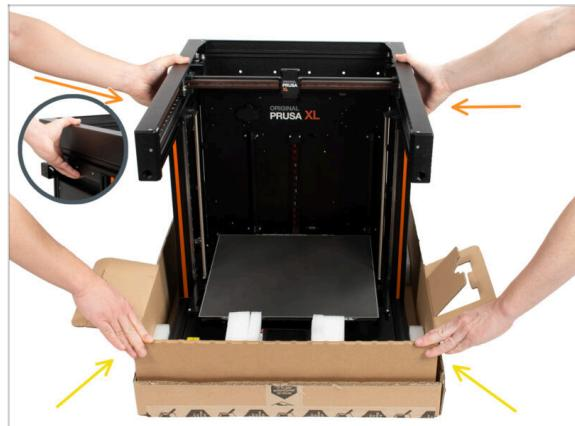
◆ Use the side handles on both sides of the printer to handle.
