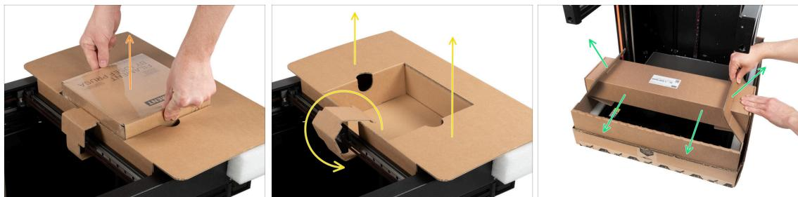
**⚠** The cardboard fixings contain the parts necessary for the assembly. **Do not throw them out!**
