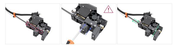
• Pull the flexible line up so that the screws engage into the narrower part of the keyhole openings.
