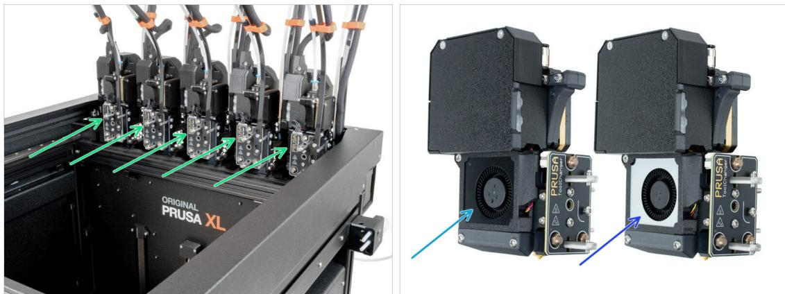
⚠ Starting January 2026, printheads are shipped with a silver print fan. Check the color of the print fan installed on the toolhead. In the following step, you will confirm the print fan type in the printer menu.
