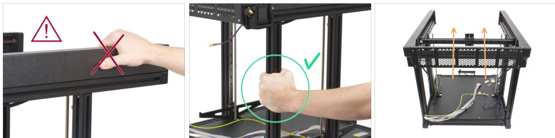
⚠ **Never manipulate the printer by using the upper metal flanges. You can damage the LED lights hidden inside.**
