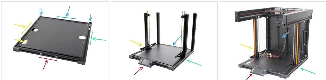
**⚠️ IMPORTANT:** Due to the XL printer's large size, it is nearly impossible to capture the entire body in each photo. Throughout this manual, specific terms will be used to describe the **side of the printer you will be working on**:
