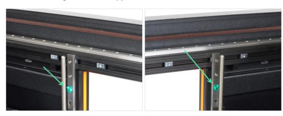
• Take off the linear rail stoppers on both inner sides of the printer.
