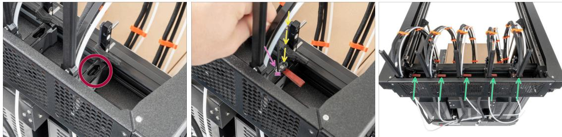
ⓘ The current nozzle seal position is temporary, the exact height will be set in the next chapter once all the Nextruder parts are mounted.
