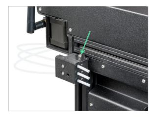
Insert the calibration pin into the left side filament sensor.
