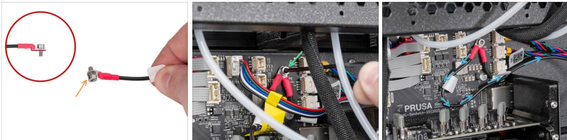
⚠ **Note the correct orientation of the PE cable connector.**
