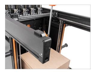
Insert the M3x10rT screw and secure it with the T10 Torx screwsdriver.
