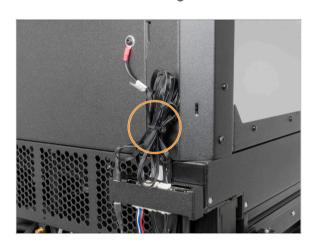
Secure all cables together with a zip-tie. Do not overtighten the ziptie. Cut the end of the zip-tie.
