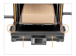
Attach the bellows on the lower belows holder with handles facing up.
