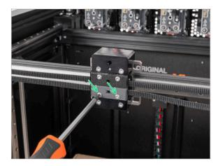
Secure the belt-clamp with two M3x12rT screws (which you removed in the previous step) with a T10 Torx screwdriver.
