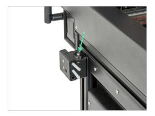
Insert the calibration pin into the side filament sensor.
