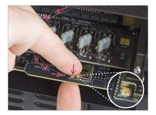
Connect the antenna to the appropriate slot on the XL Buddy board.
