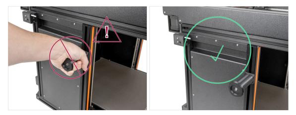
Never manipulate the printer by using the upper metal flanges. You can damage the LED lights hidden inside.
