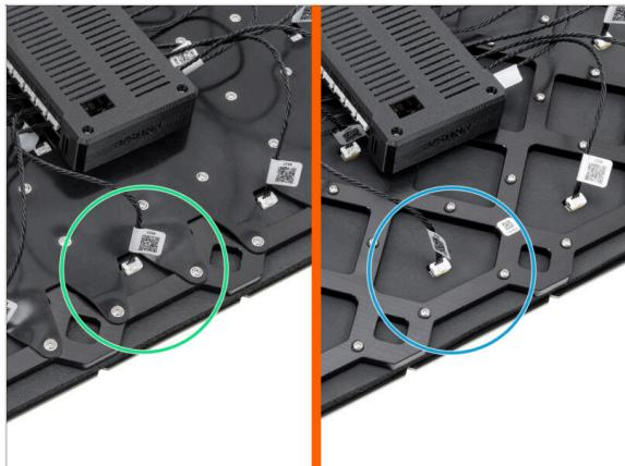
ⓘ Starting from April 2025, you may receive a new heatbed. The difference is the black rubber band on a back side of the heatbed.
