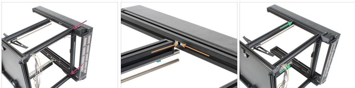
**⚠️ Be careful while attaching the extrusions and CoreXY, avoid scratching them.**
