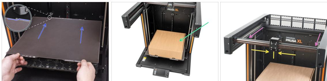
**⚠️ Reminder:** To handle the printer, **always grab the handles on both sides of the printer**. Do not lift the printer by the aluminum extrusions or the metal sheet profiles on top.
