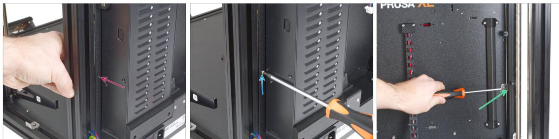
**⚠ Hold the XL rear panel with your hand during assembly! Until it is secured with screws.**
