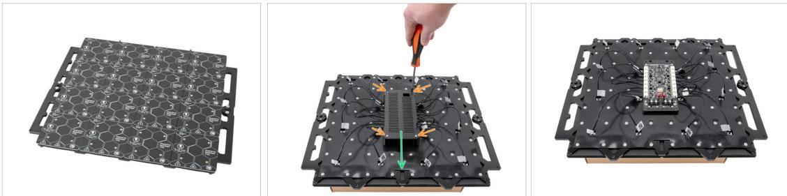
⚠️ **ATTENTION:** Make sure your workspace is clean before you start working with the heatbed. Use a soft pad underneath (cloth / cardboard) to avoid scratching the heatbed components.
