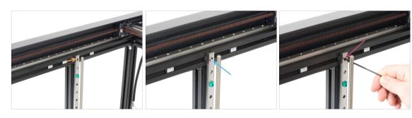
On the left side of the CoreXY, there are three M3nEs nuts in the extrusion. Slide the middle M3nEs nut behind the linear rail. Align its hole with the hole in the linear rail
