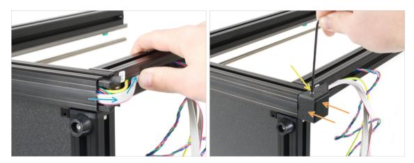
• Gently bend the cables over the corner and insert them into the extrusion. Start with the Z motor cable and then proceed with xLCD and PE cables. Gently bend the xLCD cable over the corner and insert it in the extrusion.
