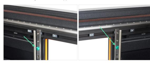
• Take off the linear rail stoppers on both inner sides of the printer.
