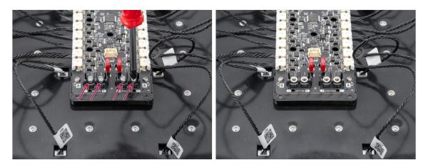
Remove the four power terminal screws using the Phillips screwdriver. **Keep them** aside as we will need them in the next step.
