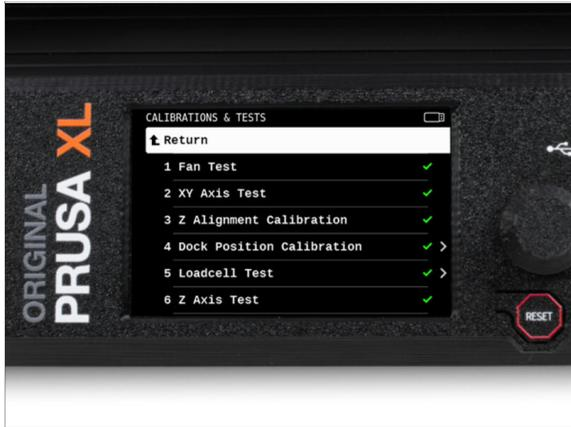
**i** The wizard will test all important components of the printer. Some parts of the wizard require direct user interaction. Follow the instructions on the screen.
