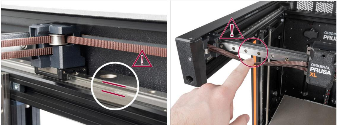
**⚠ CAUTION: Avoid direct skin contact with the lubricant used for the linear rails in this printer. If a contact occurs, wash your hands immediately. Especially before eating, drinking, or touching your face.**
