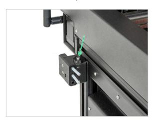
Insert the calibration pin into the side filament sensor.
