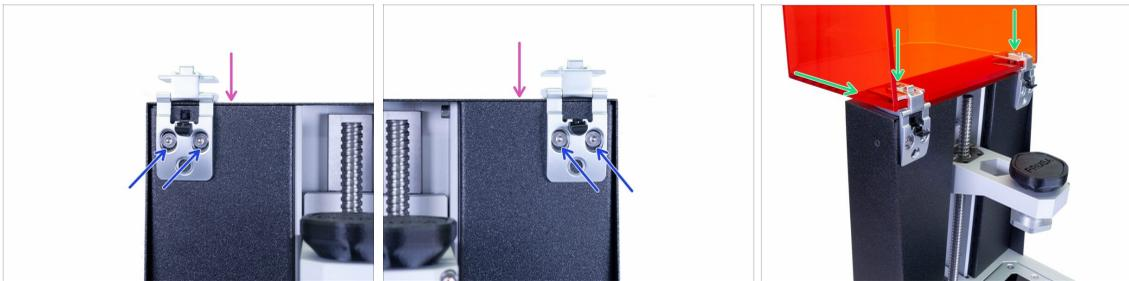
⚠ **Make sure you won't drop the hinges during the assembly. You can use any fabric to protect the FEP film and the print display below the hinges.**
