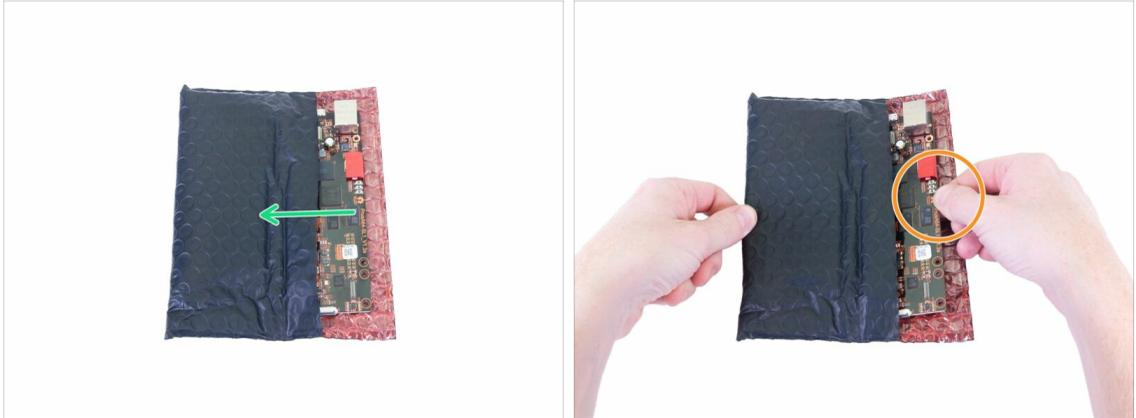
**⚠ WARNING:** Make sure to **protect the electronics against electrostatic discharge (ESD)**. Always unpack the electronics right before you need them!
