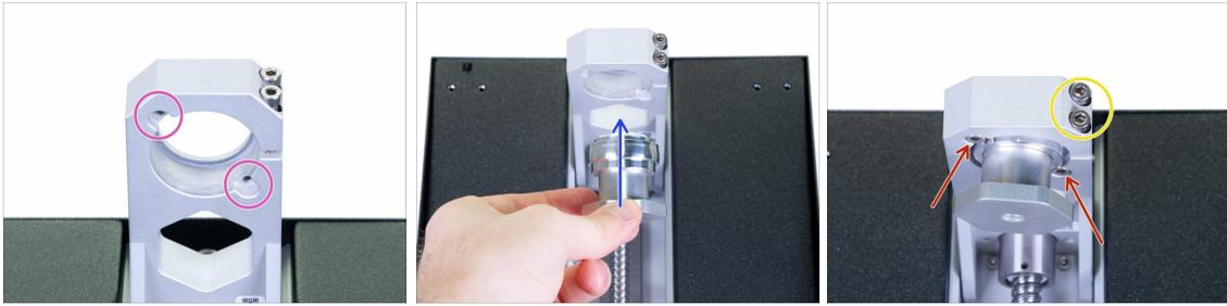
**⚠ WARNING:** This step involves inserting parts from below and it might be slightly more difficult. You can lay the printer on its back, but use the cardboard to protect the PSU power button.
