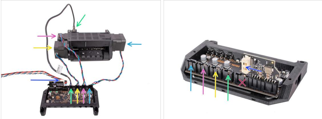
● Prepare the unit and the electronics board assembly as seen in the picture. Follow the cables to plug them in the correct order.
