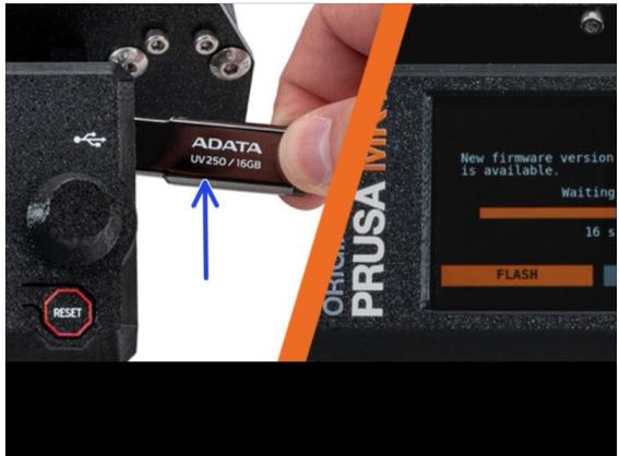
**⚠ IMPORTANT!!!** Before you proceed further; There are two firmware files. One is for the printer. The other one is for the MMU3 unit. Both needs to be flashed to the respective device.
