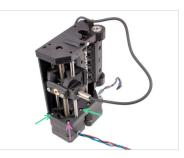
Rotate the threaded rod while pushing it towards the selector to engage it into the trapeze nut.
