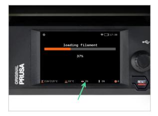
On the MK4S printer, you can check the filament sensor's status in the "footer" area of the LCD screen to see if it's detecting the filament correctly.
