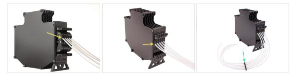
Insert the PTFE tubes into the upper collet in each of the cartridges. Push them all the way in.
