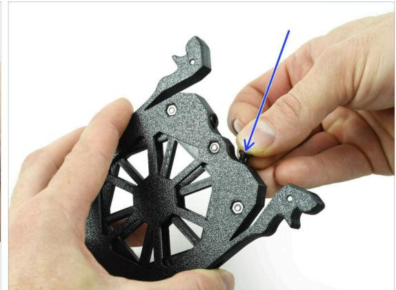
● Insert one of the **collets** into the marked position on the cartridge.
