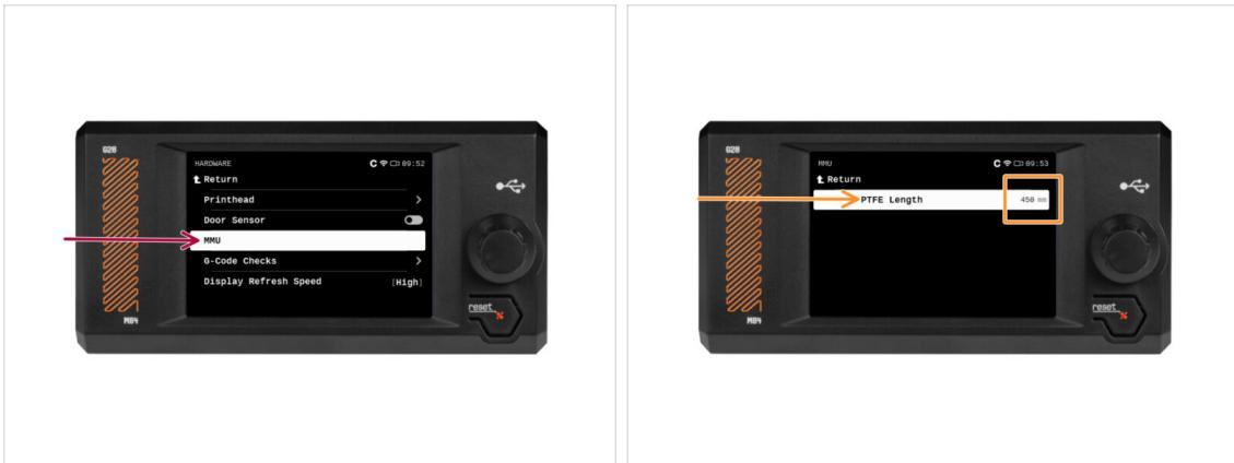
**⚠** The MMU-to-Extruder PTFE tube length needs to be set in the firmware.
