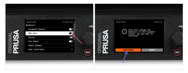
After finishing the firmware update, **make sure there are no filaments loaded** neither in the extruder, or in the MMU unit.
