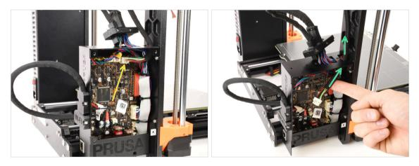
Disconnect the MMU cable from the xBuddy board. Note that there is a safety latch that must be pressed, in order to disconnect the cable.
