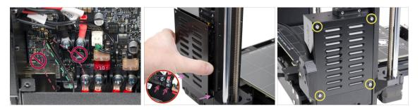
Arrange the NFC coil cable to the rightmost side as shown.
