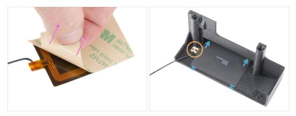
Peel of the protective layer layer from the NFCcoil.
