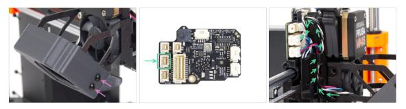
From the right side of the fan holder, secure both parts together using two M3x5rT screws.
