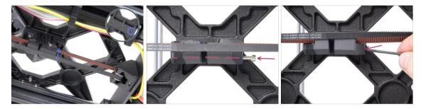
Insert the M3x10 screw into the Y-belt-tensioner and attach the Y-belt-tensioner to the right (front) hole in the Y-carriage and secure it with the M3x10 screw. Do not overtighten the screw. We will adjust the exact position later on.
