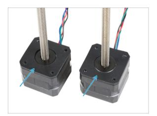
Place both rubber pads onto the motor surface. Make sure the holes in the pads are aligned with the holes in the motors.
