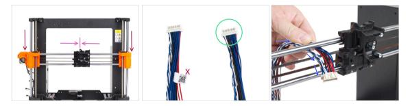
Move the X-axis assembly to the center of the Z-axis height.
