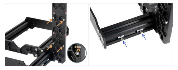
Insert four M3x6 screws to the back of the frame (side with shorter extrusions), so they resemble a rectangular pattern. Tighten the screws fully into the frame to clean the threads. Then loosen the screws, leaving a gap of at least 3 mm between the screw head and the frame.
