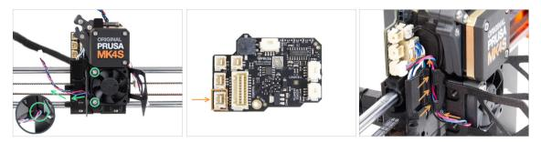
Attach the hotend fan onto the heatsink with two M3x18 screws on the left side. Tighten the screw gently, but firmly, otherwise the plastic housing may crack. The cable must be pointing towards the lower-left corner.
