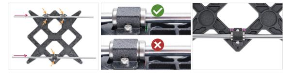
• Using a paper towel, wipe the transport oil from the surface of the smooth rods.
