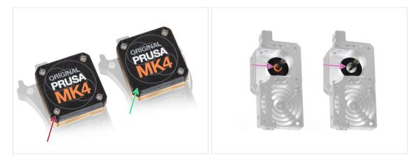
There were two types of the gearbox on the **MK4** printer.
