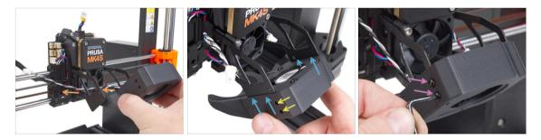
• Take the print fan blower assembly and guide the fan cable through the cutout on the left side of the fan holder.
