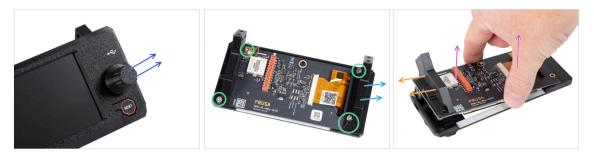
$\triangle$  Make sure the USB drive is removed from the xLCD.
