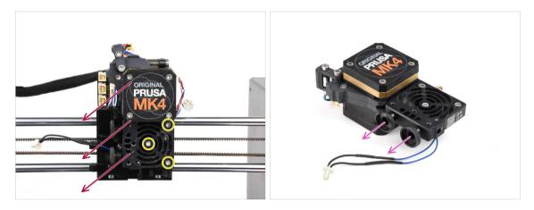
• Loosen all three M3x10 screws mounting the Nextruder assembly.
