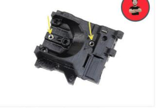
Insert two M3n nuts to the X-carriage-back.
