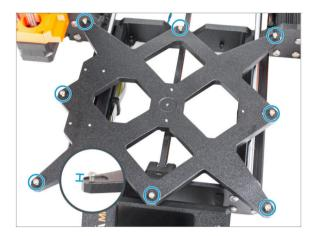
Install eight M3x6r screws in the outer holes on the Y-carriage. Do not tighten them completely. A few turns are enough for now.
