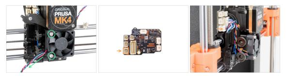
Attach the hotend fan onto the heatsink with two M3x18 screws on the left side. Tighten the screw gently, but firmly, otherwise the plastic housing may crack. The cable must be pointing towards the lower-left corner.
