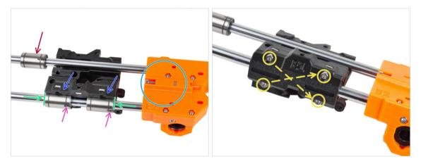
Place the X-axis assembly oriented as shown. Make sure the back of the X-endmotor is facing up.
