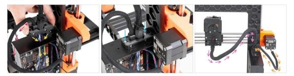
Push the X-axis motor cable and the extruder main cable through the hole in the xBuddy box to the electronics.
