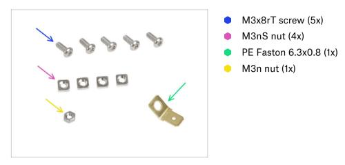
STEP 14 xLCD assembly (version B): inserting the square nuts
