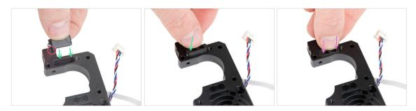
Insert the Prusa ball holder assembly into the heatsink. Make sure the steel ball part is closer to the side of the heatsink.
