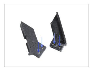
Insert two M3nS nuts into the xLCD-support-left and xLCDsupport-right.
