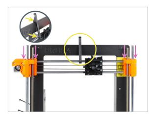
• Carefully slide the X-axis assembly onto the Z-axis smooth rods.
