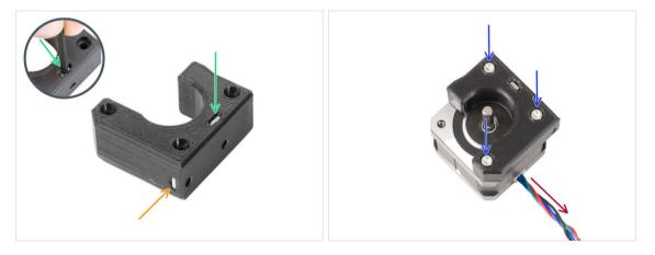
Insert the M3nS nut into the corresponding openings on the top side of the Ymotor-holder. Using the Allen key, push the nut all the way in.
