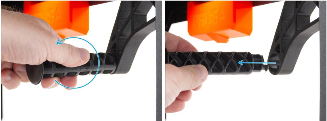
● Grasp the Spool-holder-r and turn clockwise to unlock it and remove it from the MINI Enclosure.
