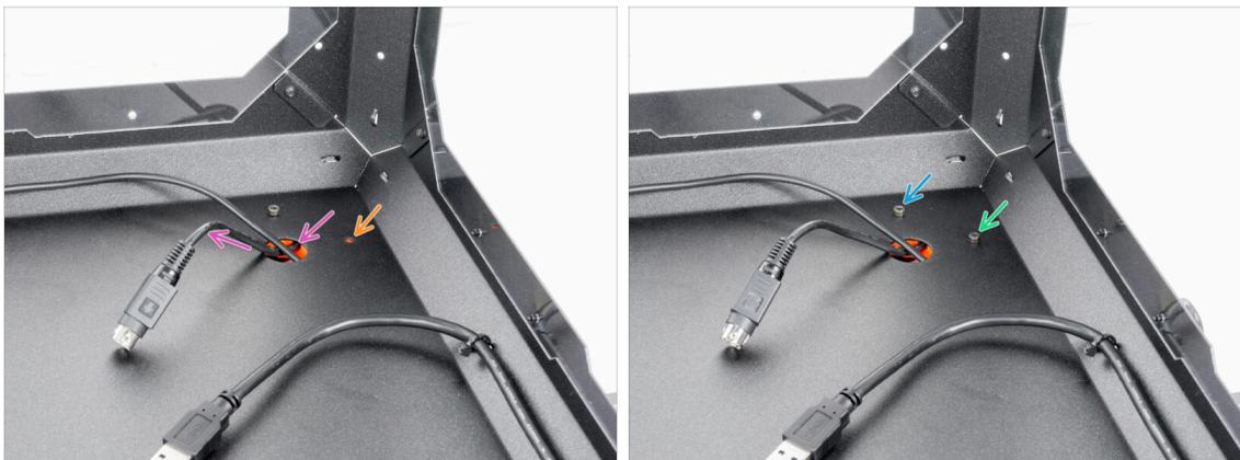
➤ Insert the printer PSU cable back through the rear hole.
