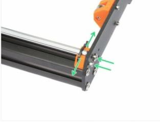
**⚠ IMPORTANT:** proper alignment of the smooth rods is crucial to reduce noise and overall friction.
